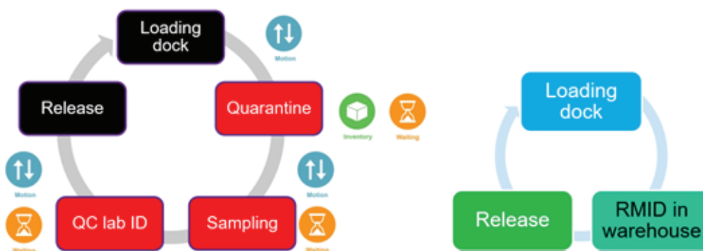
Fig. 1: Traditional RMID process cycle (left) compared to RMID performed in the manufacturing area (right), kept to a minimum.
