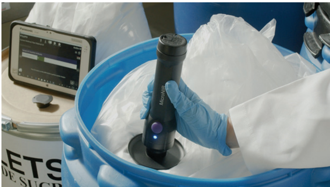
Fig. 4: The sampling collar, single push-button operation, rapid measurement cycle, and lightweight of the MicroNIR OnSite-W minimize sampling errors and fatigue. Results are displayed rapidly on the Bluetooth-connected tablet PC.
