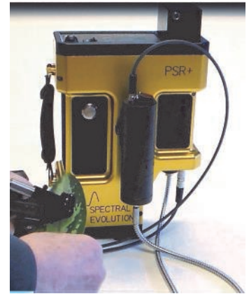
The PSR+ field spectroradiometer and leaf clip can be used to measure water content in leaves.
