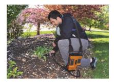
Our spectroradiometers are designed for field use: rugged, lightweight, battery operated. Our unique leaf clip includes an integrated light source and built-in reflectance standard for ease-ofuse and keeps your sample away from heat.
