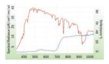
Reflectance of grass field section measured using the PSR-1100f with a standard 4° field of view lens. Red trace represents a control solar scan as measured from a reflectance panel. The blue trace represents a scan of the grass.
