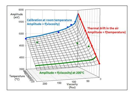
FIGURE 10. 3D FIT WITH CURRENT DRIVE
