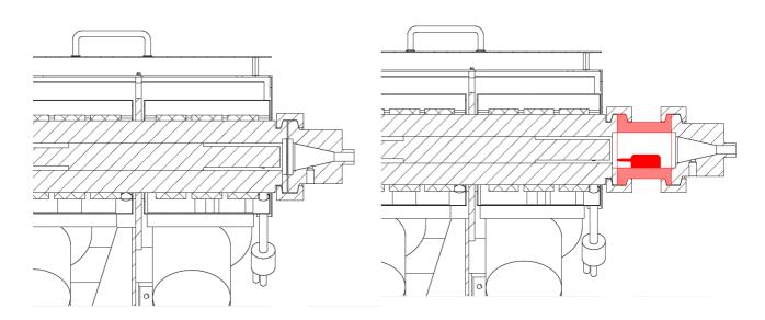
FIGURE 9. ILLUSTRATION VERY HIGH VISCOSITY SENSOR MOUNTING ON EXTRUDER
