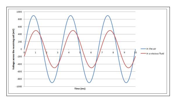
FIGURE 3. AMPLITUDE DIFFERENCE IN AIR AND IN VISCOUS FLUID
