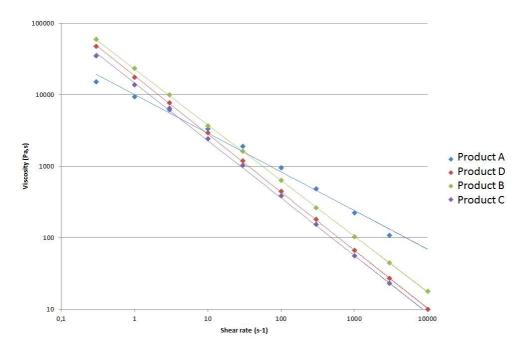
FIGURE 15. PRODUCTS A, B, C AND D VISCOSITY VS SHEAR RATE ON LABORATORY RHEOMETER
