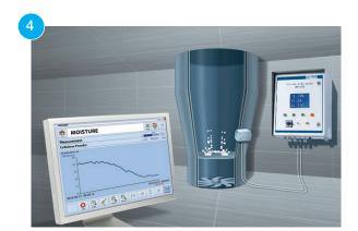
4. The instrument continuously calculates and displays the actual moisture values. Readings can be monitored online via an attached PC and also are available e.g. for a PLC.
