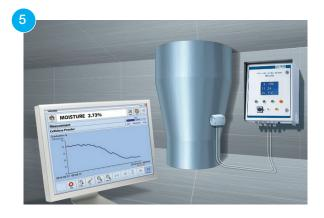
5. The moisture of the granules can be monitored during the drying process - without taking samples and without waiting for results.
