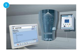
On the sensor's front surface a low-energy microwave field is generated which penetrates the granules. The instrument measures and analyzes the field's interaction with the water molecules.
