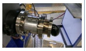
Measured in line viscosity with Soflux (at about 1 000 s $^{-1}$ ) of 245 Pa.s, correlated to the lab measurement at 1 s $^{-1}$  of 10 208 Pa.s
